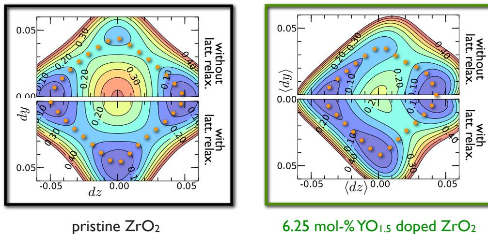
**Figure 2:** Potential-energy surface for pristine zirconia  $\text{ZrO}_2$  (left) and Yttria-doped  $\text{ZrO}_2$  (right). In the upper panels, lattice degrees of freedom are not accounted for, while in the lower panels they are. Adopted from reference [2].
