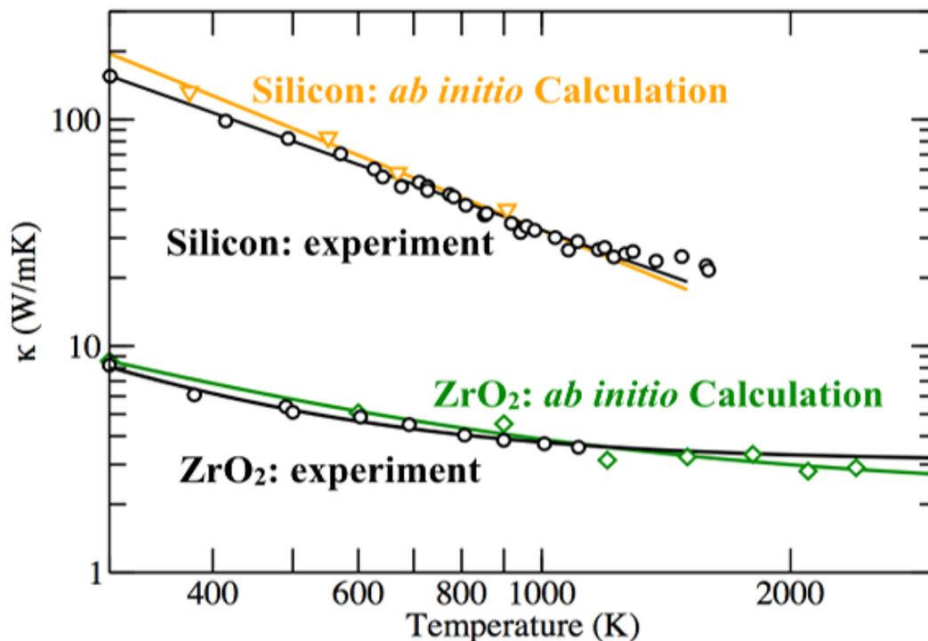
**Figure 1:** Thermal conductivity of silicon (heat conductor) and zirconia (ZrO<sub>2</sub>, heat insulator) as computed from first principles. Adopted from reference [1].
